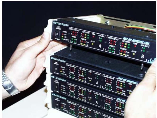
“Stacking” the Lincs distributes power up from the base to the Lincs via the power jacks on each module from the receptacles below. Align the tips of the jacks with the center of the receptacles’ openings on the Linc below.
